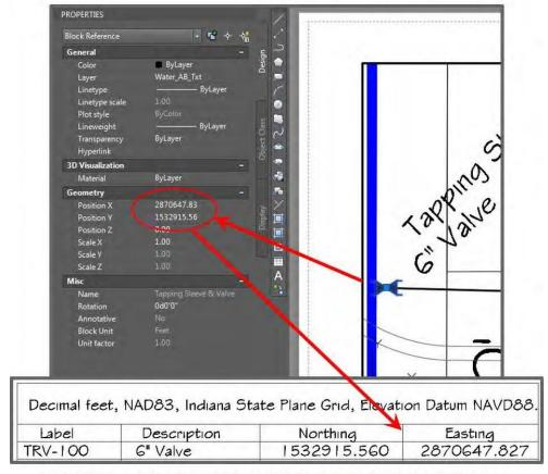
This example shows how the valve drawn in the correct coordinate system will display the same coordinates as the Northing and Easting Table. All tie in locations (tapping valve, sleeve, etc, will have Northing and Eastings in table format and be accurately drawn on the map.
